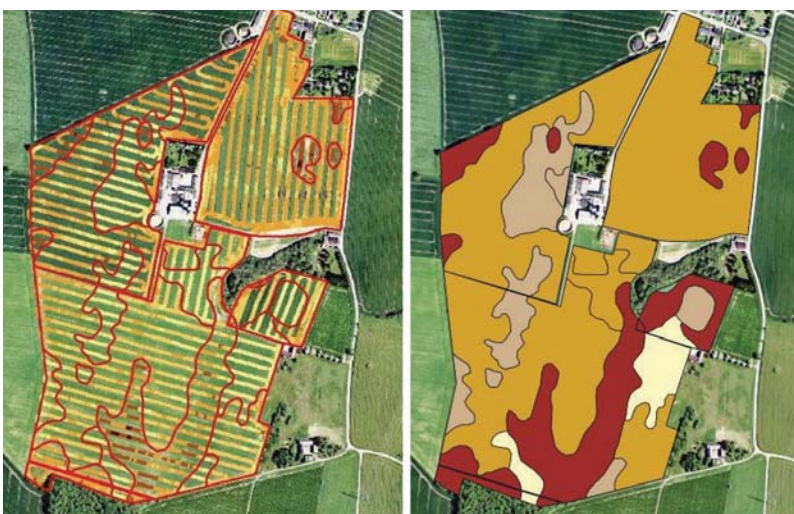
Figure 3. The map at left shows the results of measurements with the EM38 technique and classical methods, from which the final soil maps (right) are produced. Colours in the map to the right represent different clay contents, where white = 0-5%, grey = 5-10%, yellow = 10-15% and brown = >25%.
