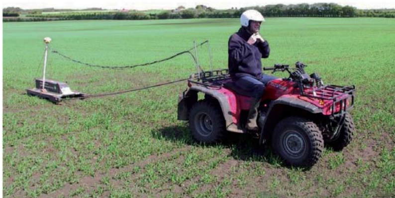
Figure 1. Apparent electric conductivity is measured using an EM38 sensor mounted on a sledge.
